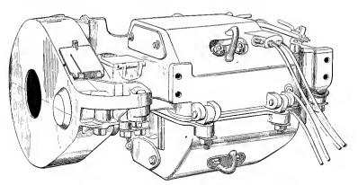
FIG. 142. View of series railway motor, closed (G. E. Co.).
